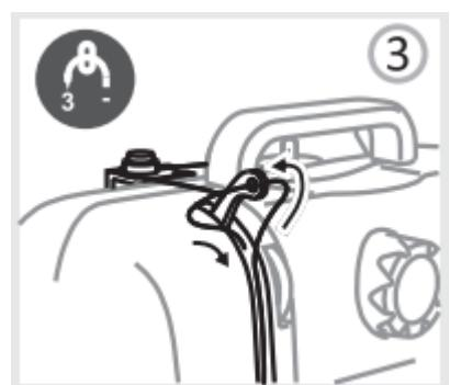
4. Go through the hole next to the needle clamp screw from up to down.
